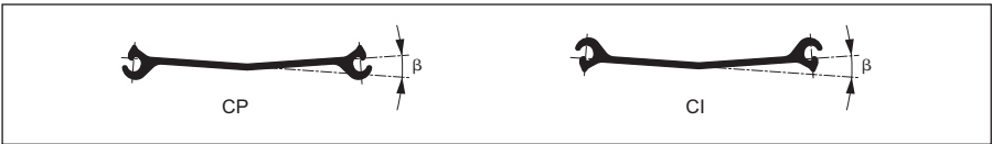
Fig. 10.3. AS 500 bent piles.
