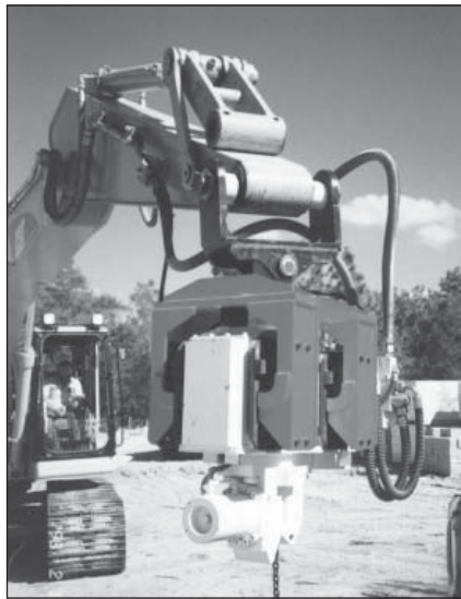
Fig. 11.14. Excavator mounted with vibratory hammer.
