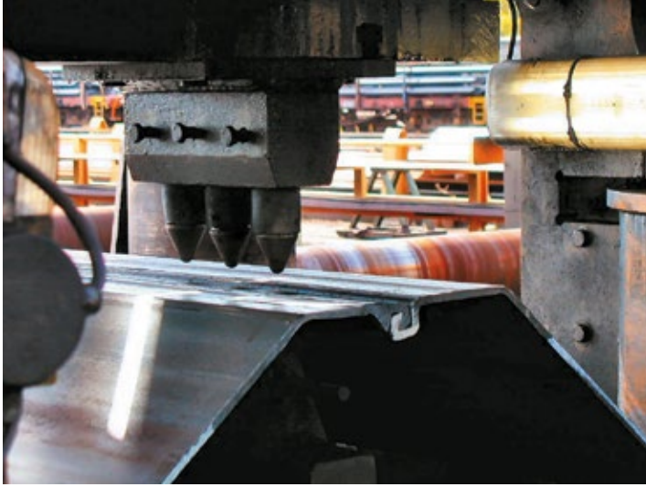
1) Amount and layout of crimping points may differ at both ends. Special crimping on request.
