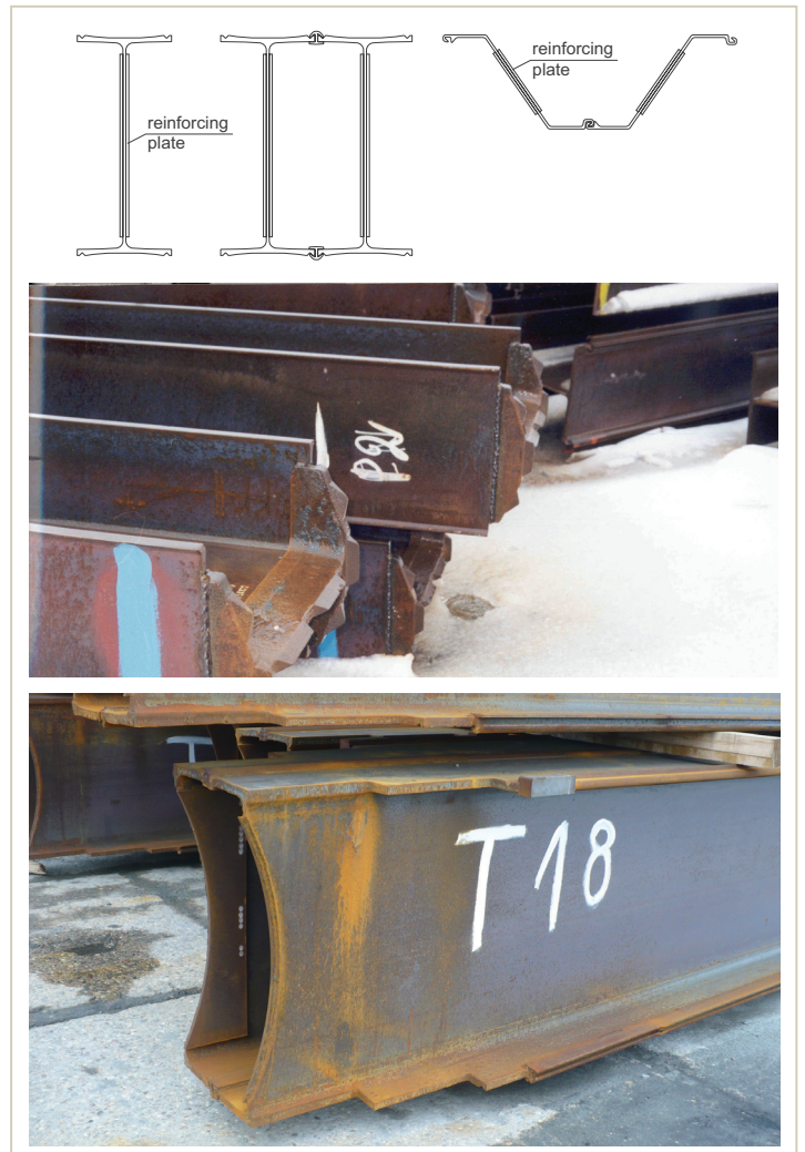
Fig. 17. Reinforcing of the tip of the pile with steel plates / shoes welded on the king pile toe.
